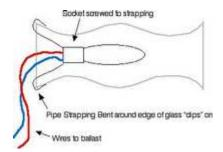
In the graphic, a length of pipe strapping bent in a "U" shape is used to hold the socket far enough inside the glass to place the bulb roughly in the middle of the glass. This glass, \$3.99 at Hobby Lobby, is 11 3/4" long and 4 5/8" at each end. Notice this glass is symmetrical. Don't try to use the asymmetrical hurricane lamp "chimney's" available at Lowe's or HD; they're too small and aren't shaped in a way that permits good air flow.
