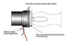
This will allow us to use a 5" hose clamp to secure the edge of the reducer collar to this tape wrapped "cushion." (Note: you can use foil tape alone for building this "cushion" but the thermal wrapping makes for a neater seal, and is less susceptible to heat. Also, if a hose clamp isn't available, the reducer can be secured to the glass with foil tape.
