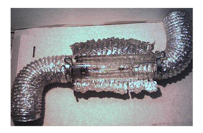
A couple of wraps of pipe wrap sealed with foil tape on each end you want to put a collar on should be used to keep from biting the metal directly into glass with the hose clamp (pictured). The socket is mounted inside the tube with pipe strapping just as in the hurricane style fixture. It can either be "clipped" and taped over the edge of the glass or better, pop riveted to the inside of the starter collar.
