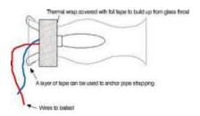
The wires from the socket can be either run through your 4" ducting which will attach to the other end of the reducer or you can drill a hole in the tapered part of the reducer to run the wire out of the fixture to the ballast.
